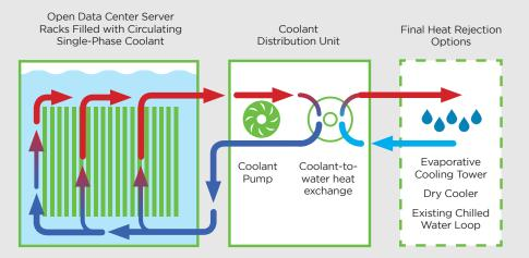
Heated coolant exits top of rack. Coolant returns to rack from heat exchanger at user-specified temperature.
