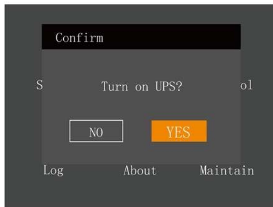
Figure 5-5 Switching the UPS on
